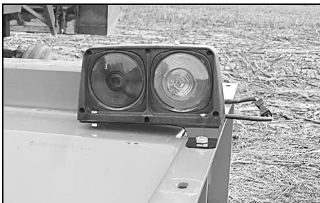
Figure 50. Safety Light Installed - Rear View
